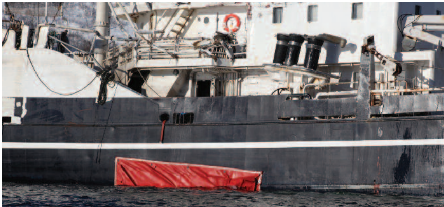
The refloated Hundvaky , with a temporary patch clearly visible
